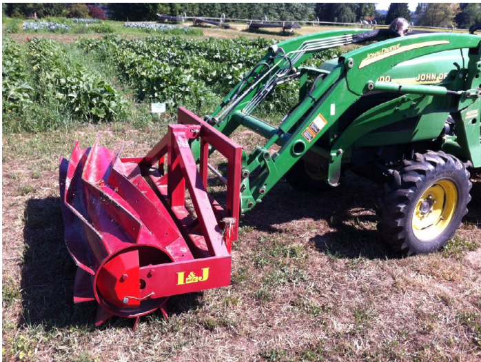
Image 3. The roller crimper is used to terminate a cover crop and leave it as a mulch on the surface.
