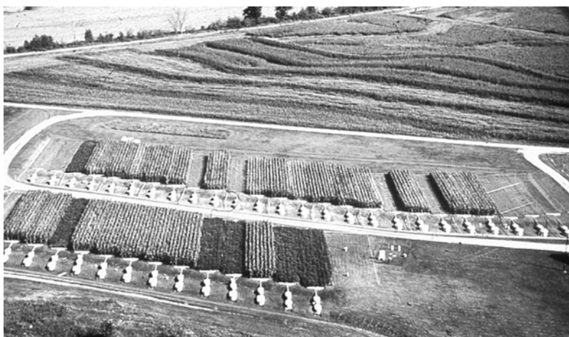
Figure 5.6. Erosion plots 12 ft wide (3.65 m) and 72.6 ft (22.1 m) long near Columbia, MO.
